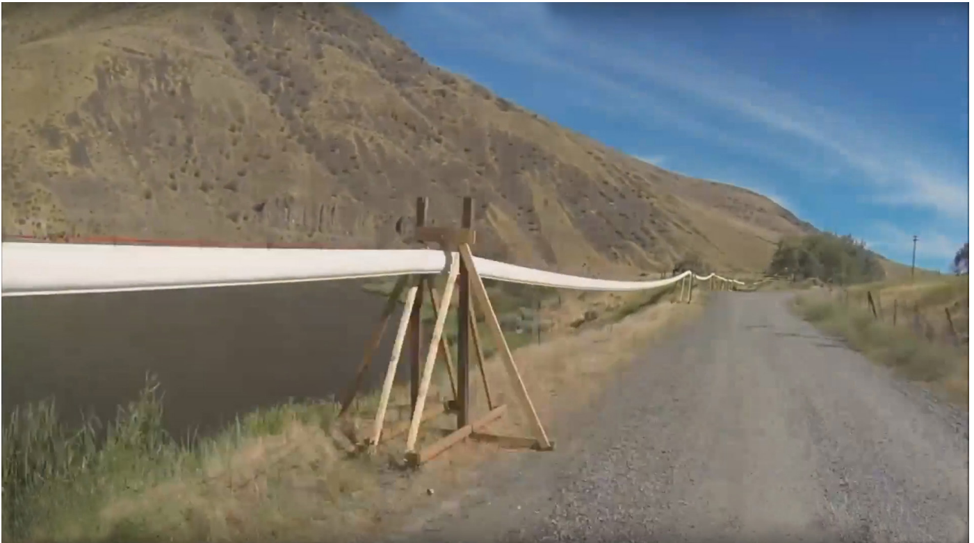
Figure 4: Absurdity via Intensification: In a feasibility study, Whooshh tests the limits of the Salmon Cannon extending its run to over 1000 feet, almost twice its typical distance.
