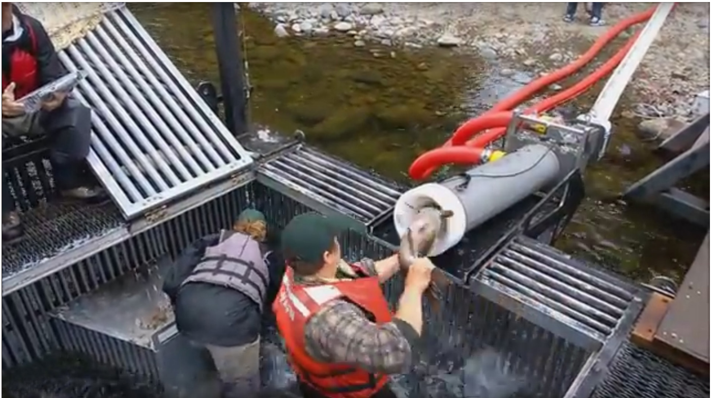
Figure 1: Entangled Imaginaries: Fish traveling upstream are inventoried in a mechanical enclosure before human handlers manually guide them into the induction tube of the Salmon Cannon.
